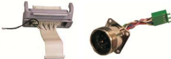
6. Reconnect the encoder cables to EXE 932: Y to X3; Z to X2; X to X1.
